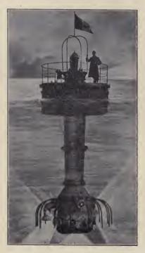
Hydroscope invented by Pino for exploring the sea bottom and successfully used in finding the galleons of Vigo Bay.
